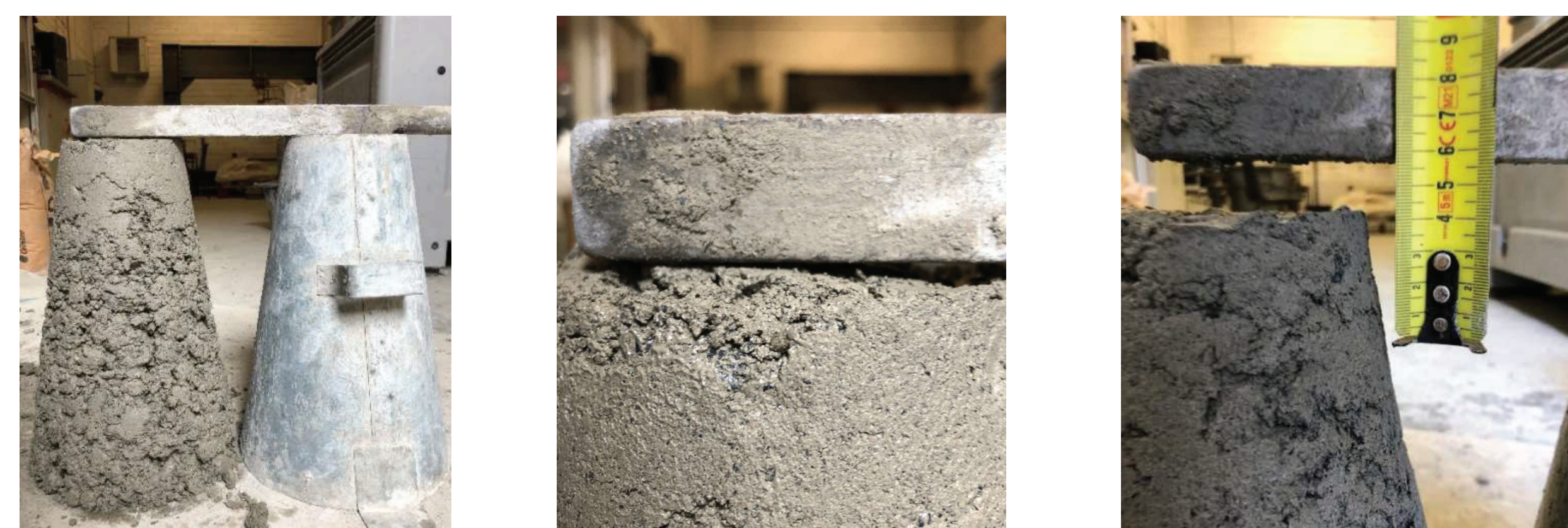
Stiff, dry slumps indicate low workability in fresh LC 3 concrete
