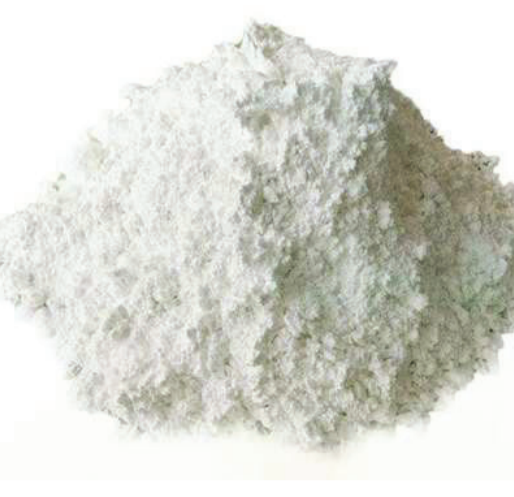
Limestone A filler in cement that accelerates cement hydration
