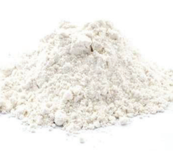
Gypsum Regulates the setting time of cement
