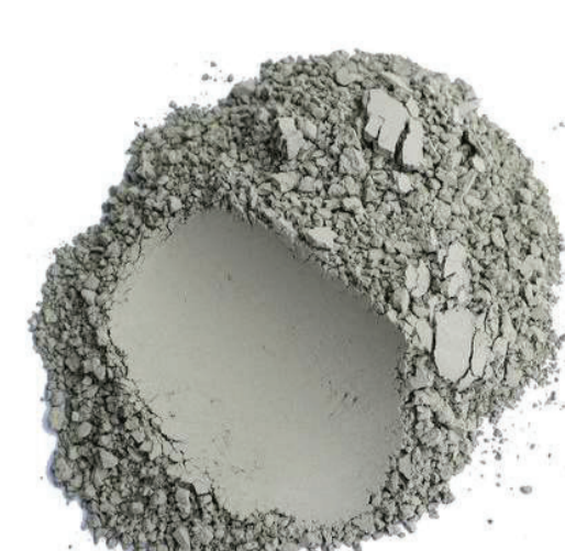
Clinker The binding agent of cement
