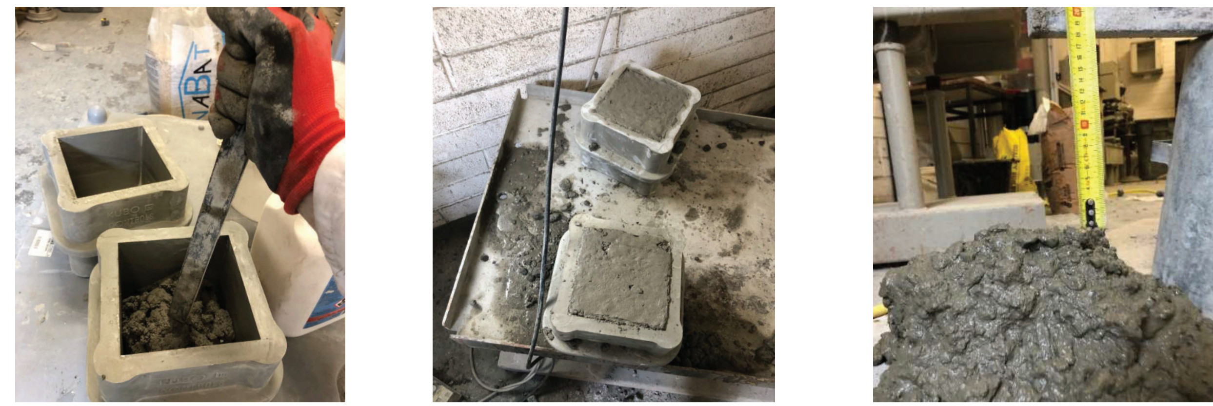
Low workability = extensive and energy-intensive compaction into cube moulds
