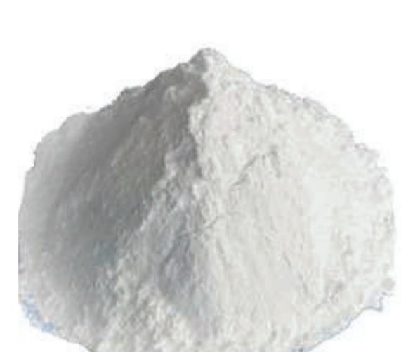
Calcined clay A pozzolanic material that can reduce clinker content in cement
