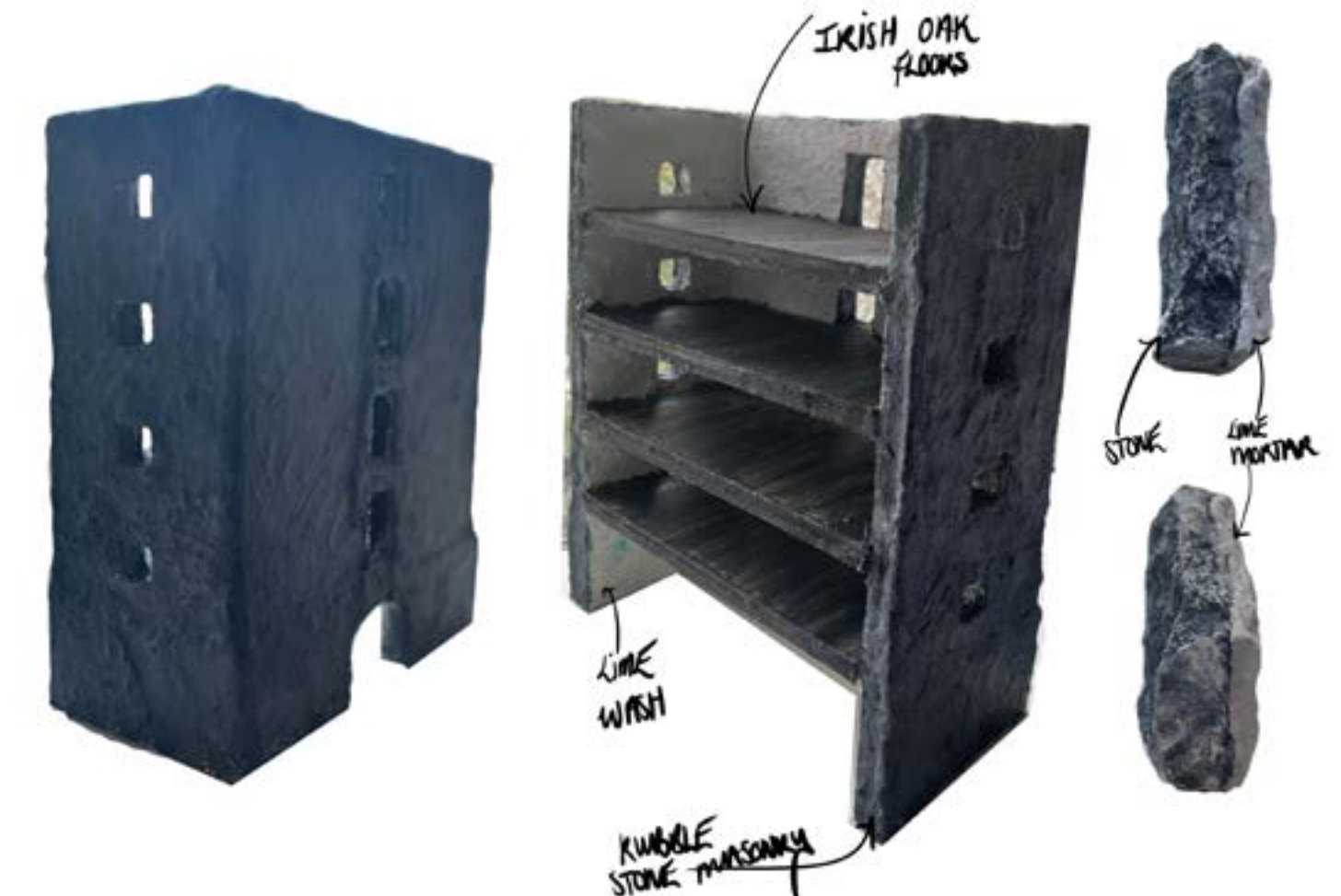
Figure 40: Models of the original Mill replicating the dense rubblestone masonry, lime wash render & Irish Oak floor
