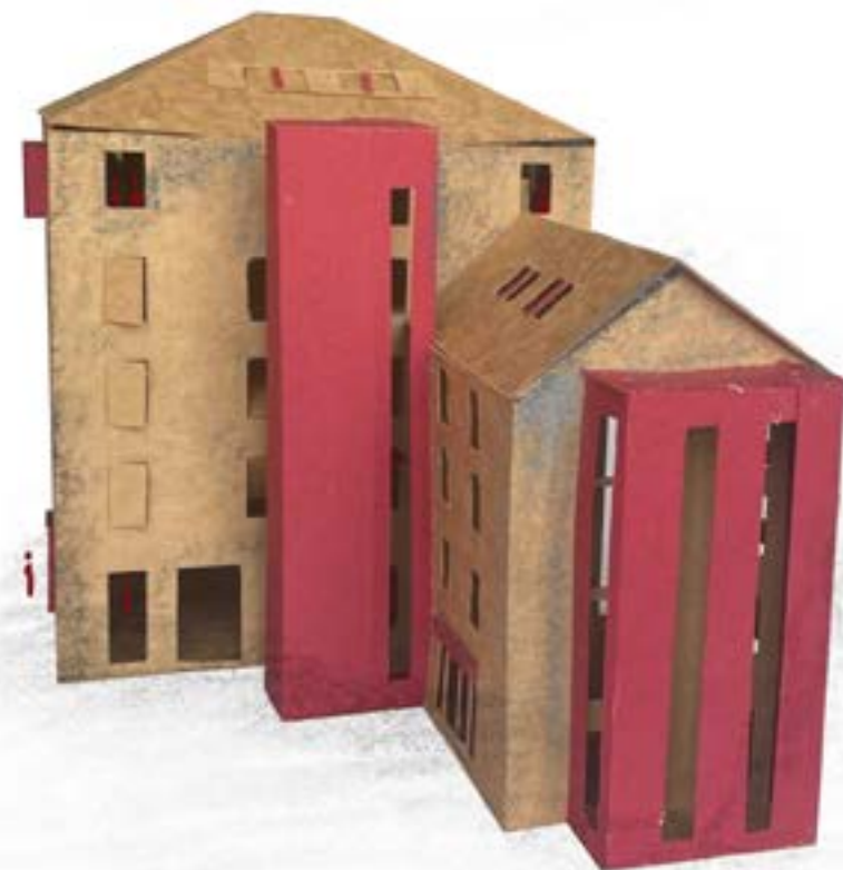
Model of new insertions and changes (red) to Mill to cater for 21st century industry/ change of
