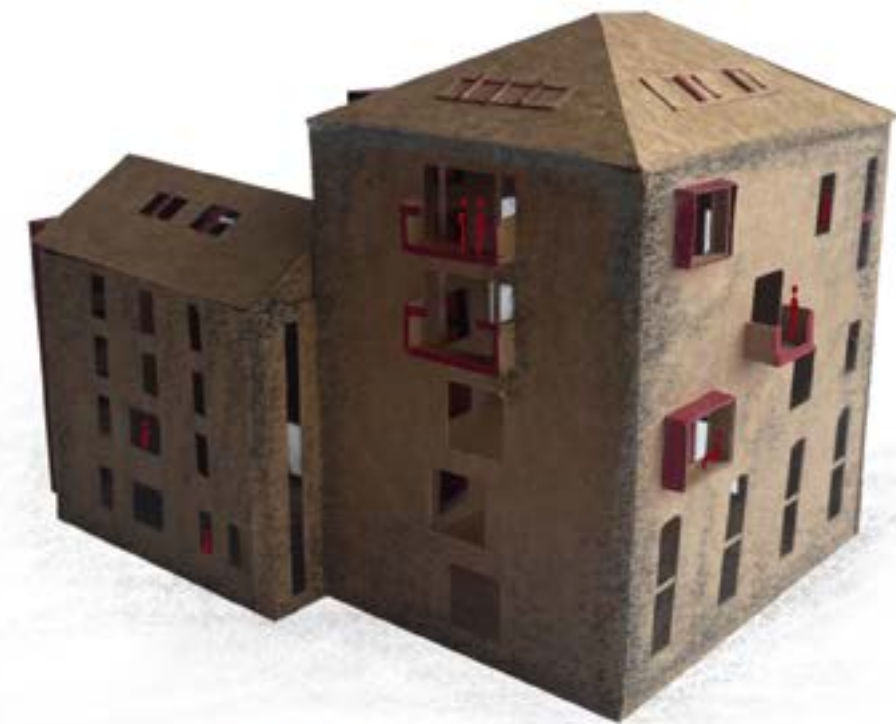
New rooflights & larger openings: increased natural light & ventilation
