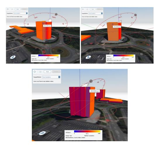
The results show the yearly cumulative value in Kw/h of solar radiation received on each facade. The south-west facade receives 682 Kw/h/m2, the south-east facade receives 735 Kw/h/m2 and the north-west facade receives 283 Kw/h/m2.
