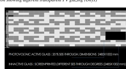
Elevation showing different transparent PV glazing (Onyx)
