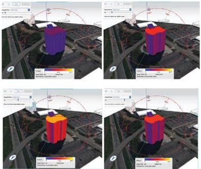
The results of the FormIt simulations, which assessed the solar exposure in kWh yearly cumulative for the case study building, were used in manual calculations to estimate the potential
