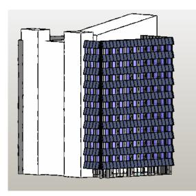
The Revit model of the case study building was not only used for showing integration of PV glazing but also for daylighting simulations.
