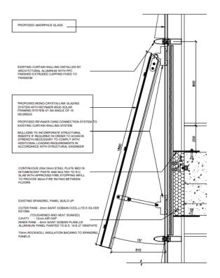
The amorphous units were integrated into the building envelope by recladding the existing glazing. The amorphous units have a upgraded U-value of 1.2W/m2K.
