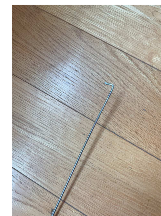
Clothes hanger end used for taking the measurements inside wall, inserted into wall, hooked onto various materials with measurements taken. Polystyrene insulation was pulled out of the wall in
