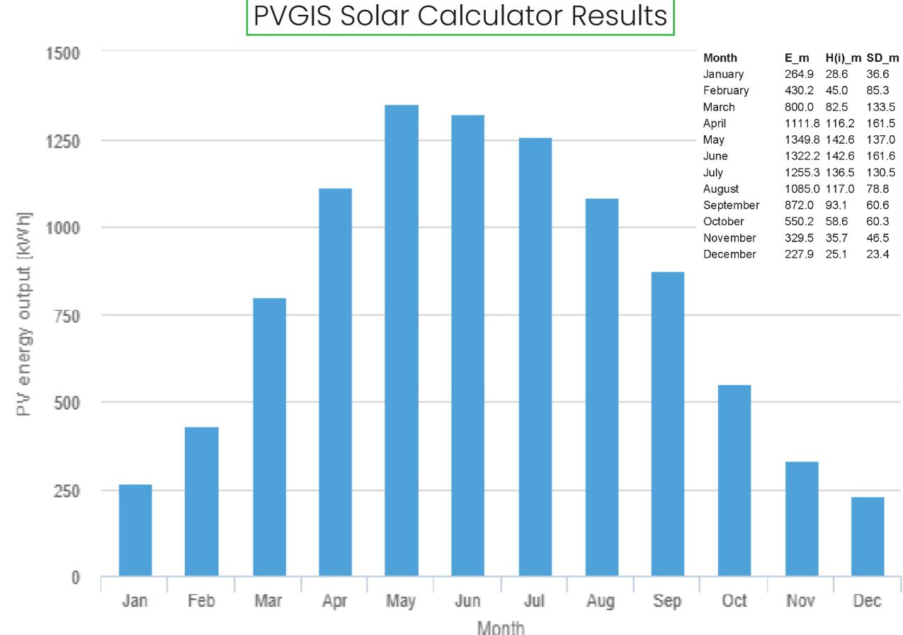
With the implementation of Solar PV Panels to the Retrofit scheme of Liberty Hall, a PV energy production of 9598.69 kWh is predicted per annum. This amount of energy that is being saved is equal to:
