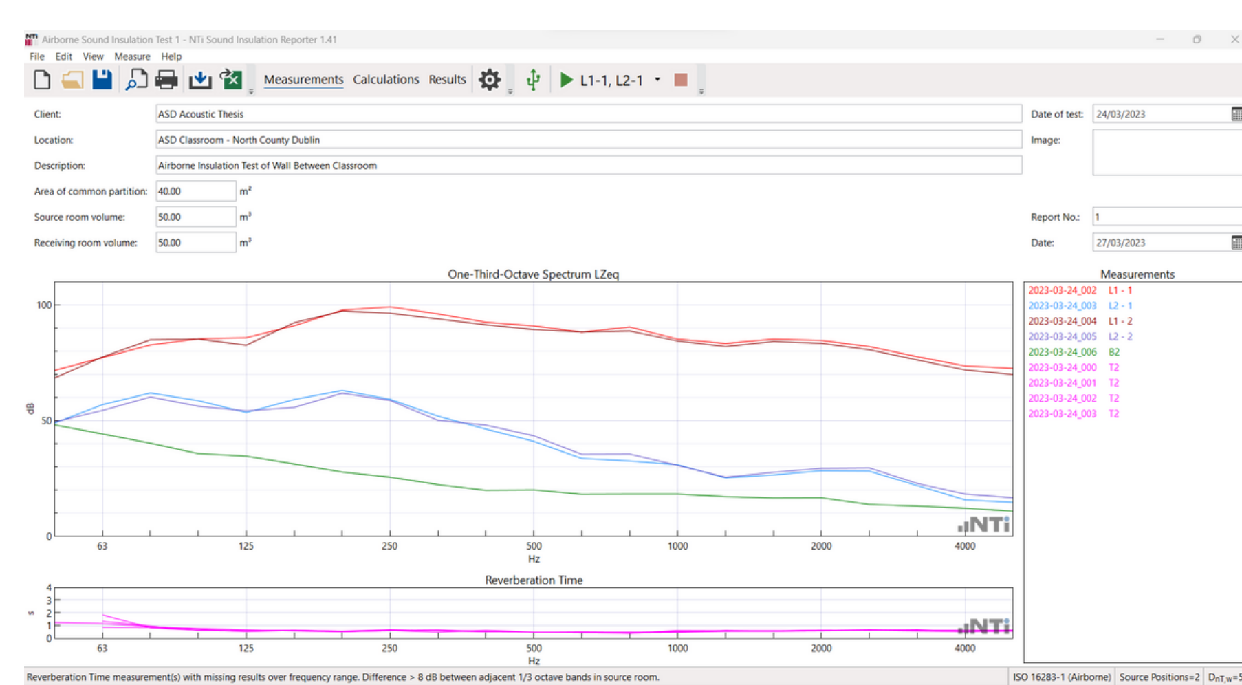
Step 5 - Input Sound Measurements into the NTI Sound Reporter Software to Calculate Results
