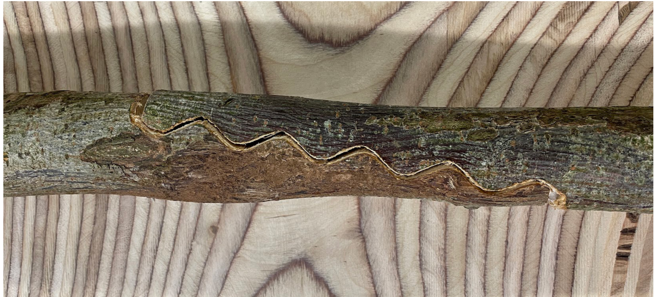
Figure 6.05: Modified Scarf Joint Tested At 1:1 Scale | Nolan | 2022
