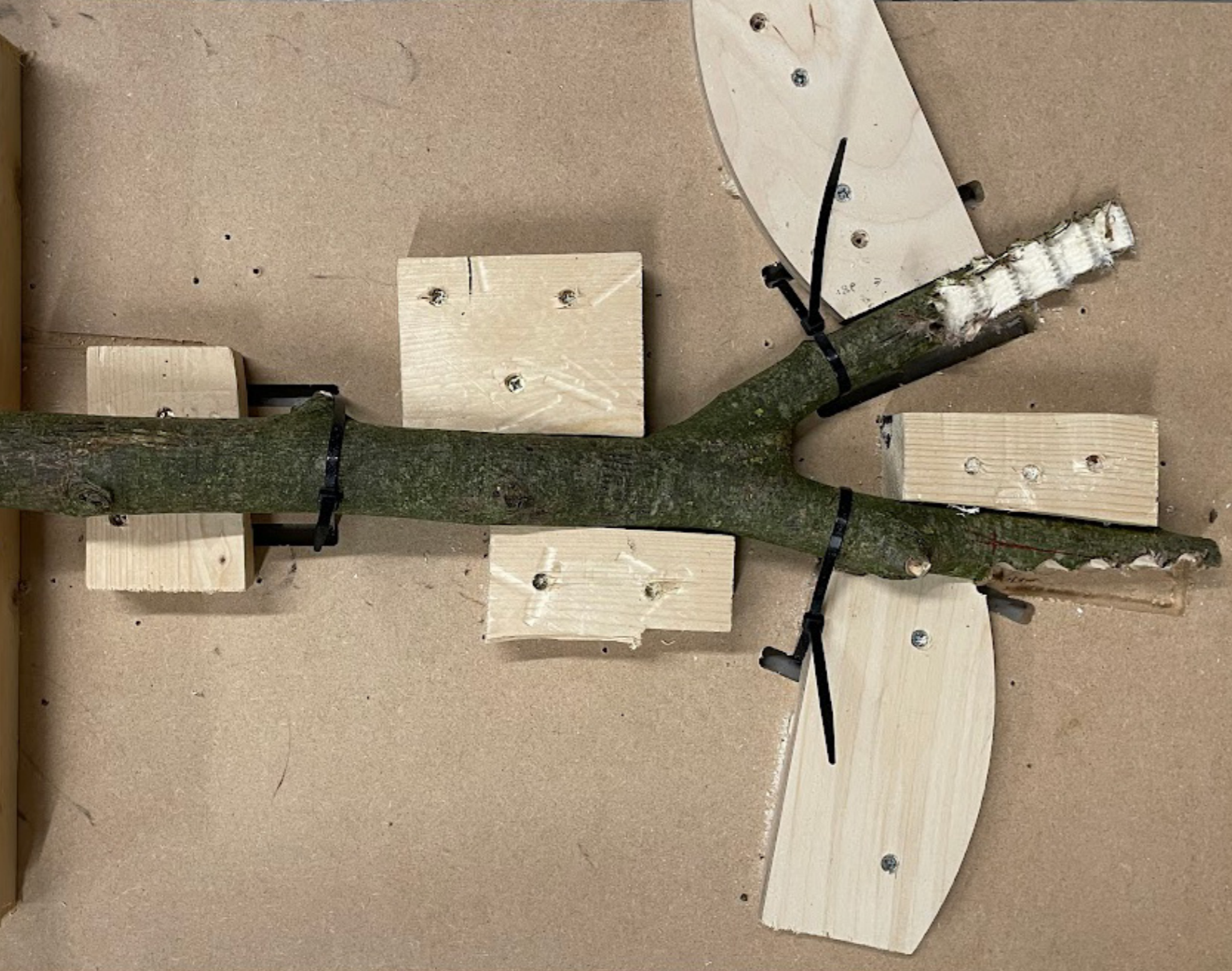
Figure 6.03: Jig for CNC Machine In Order To Hold Branch In Position | Nolan | 2022
