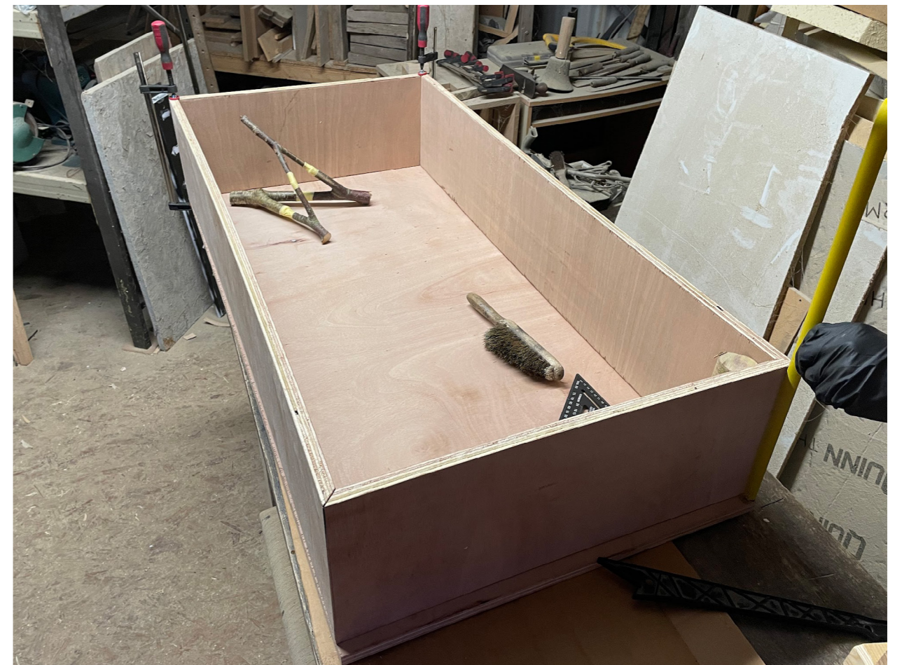
Figure 10.03: Assembling of the top carcass for the display Cabinet | Nolan | 2023
