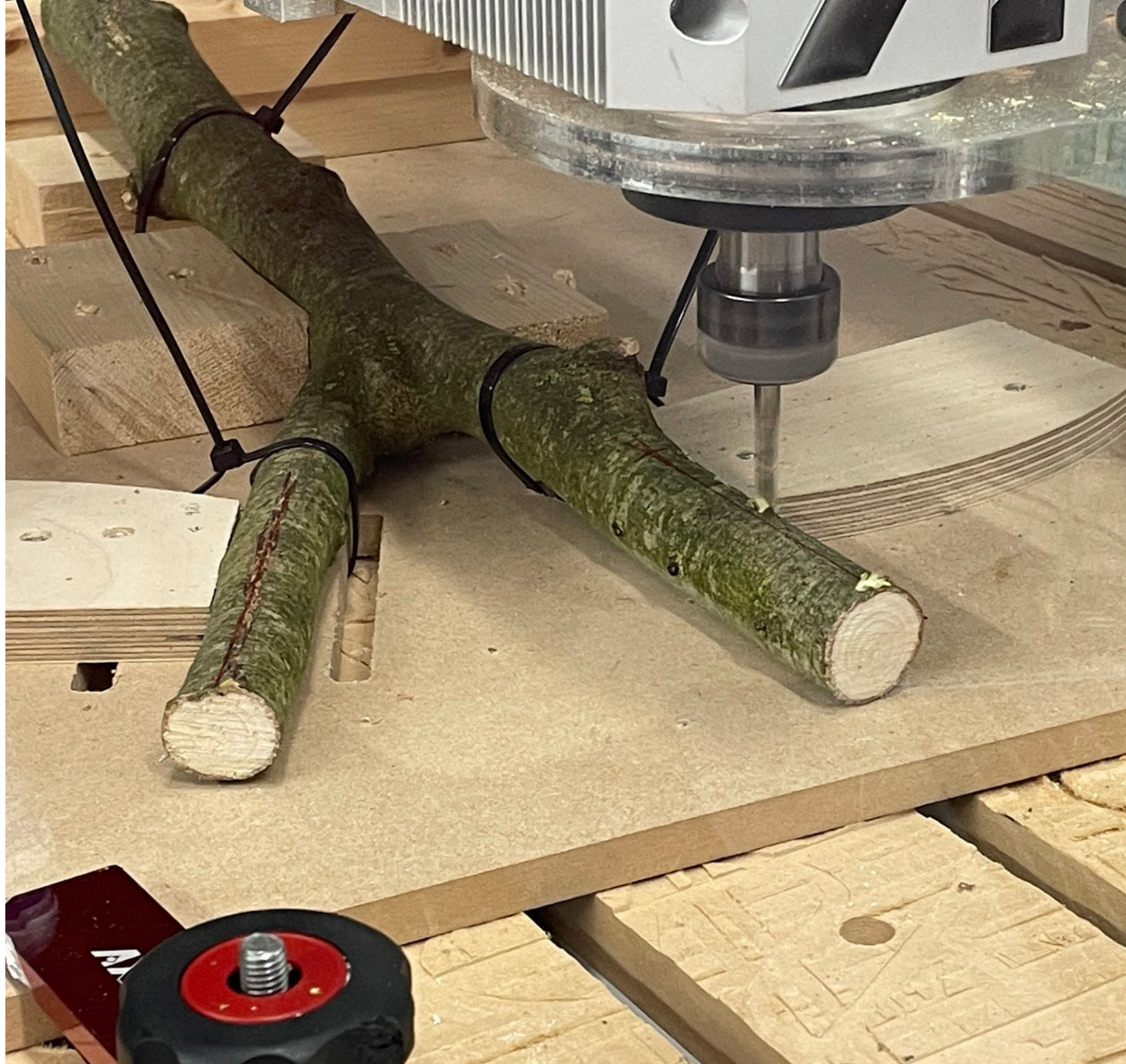
Figure 6.02: Forked Branch Having the Connection Joint Cut into it by the CNC Machine | Nolan | 2023
