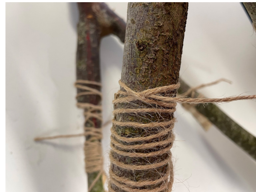
Figure 6.12: The Flax acts like a sleeve around the two branches | Nolan | 2022
