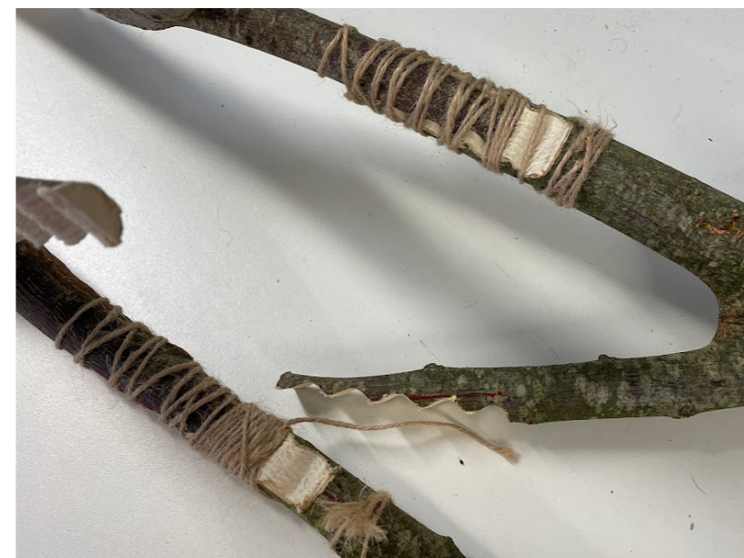
Figure 6.13: View from above of the Modified Scarf Joint bound with Flax Rope | Nolan | 2022
