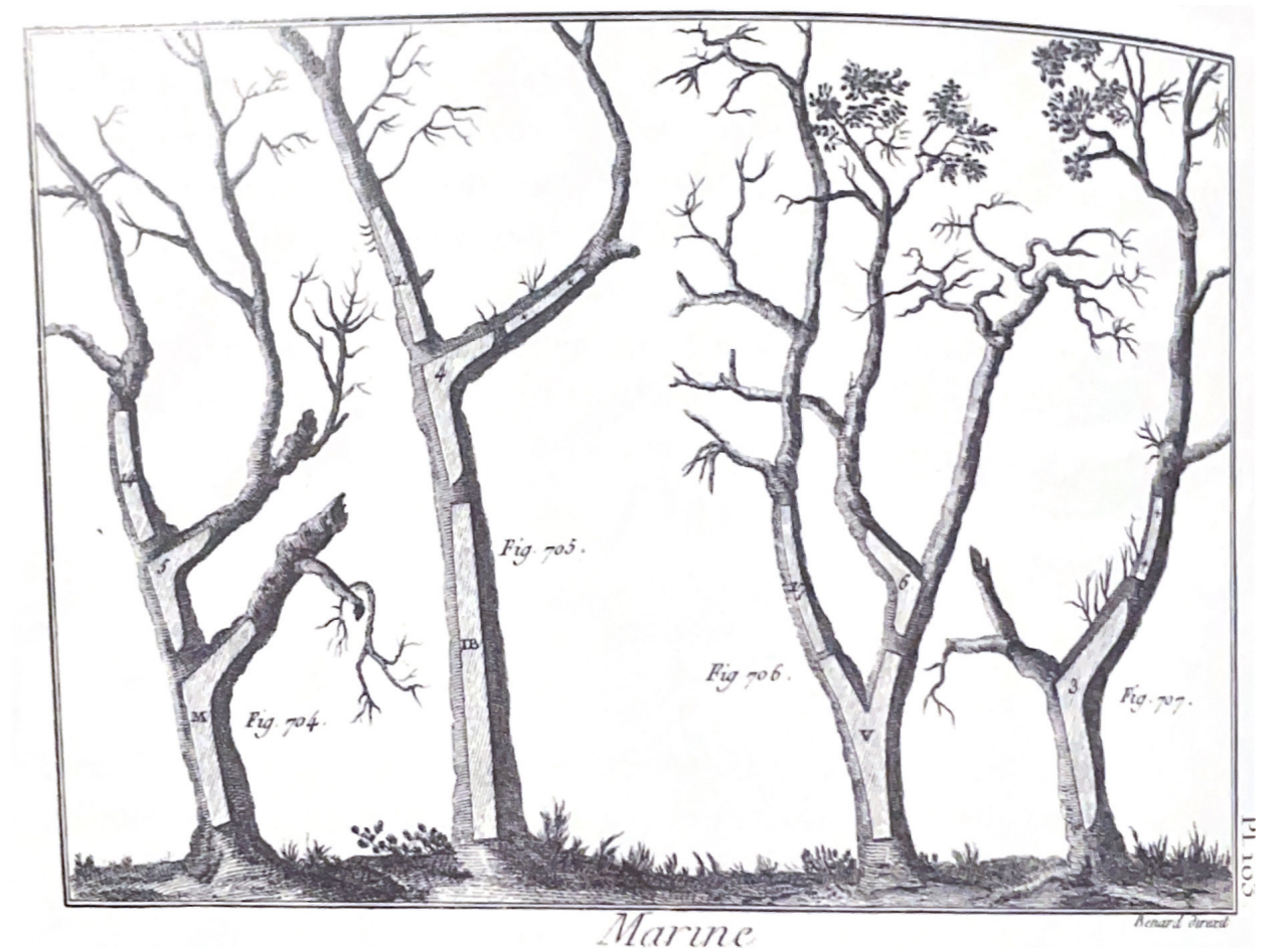
Figure 2.02: Natural-form timber elements for Ship Building | Marine | 1798
