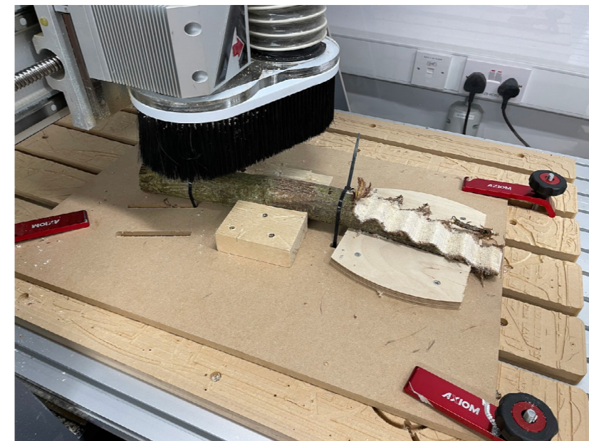
Figure 6.08: Initial Test of the Final Wave That Was Cut Into the Branch at a Scale Of 1:1 | Nolan | 2022
