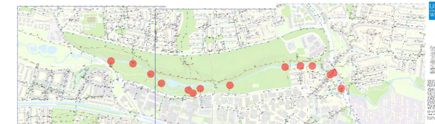
Figure 1 Drainage maps acquired from Dublin City Council for Tolka Valley Park and its surroundings. Surface runoff outfalls highlighted in red.
