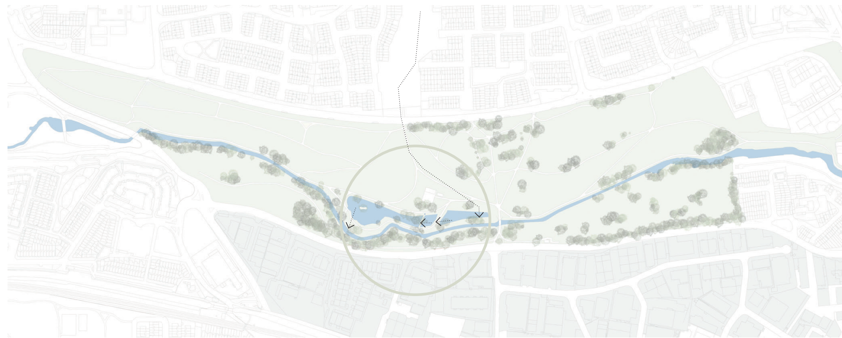
[fig 23] (left) Location plan of Tolka Valley park. Wetland highlighted with path of culverted outfall for treatment before entering the River Tolka
