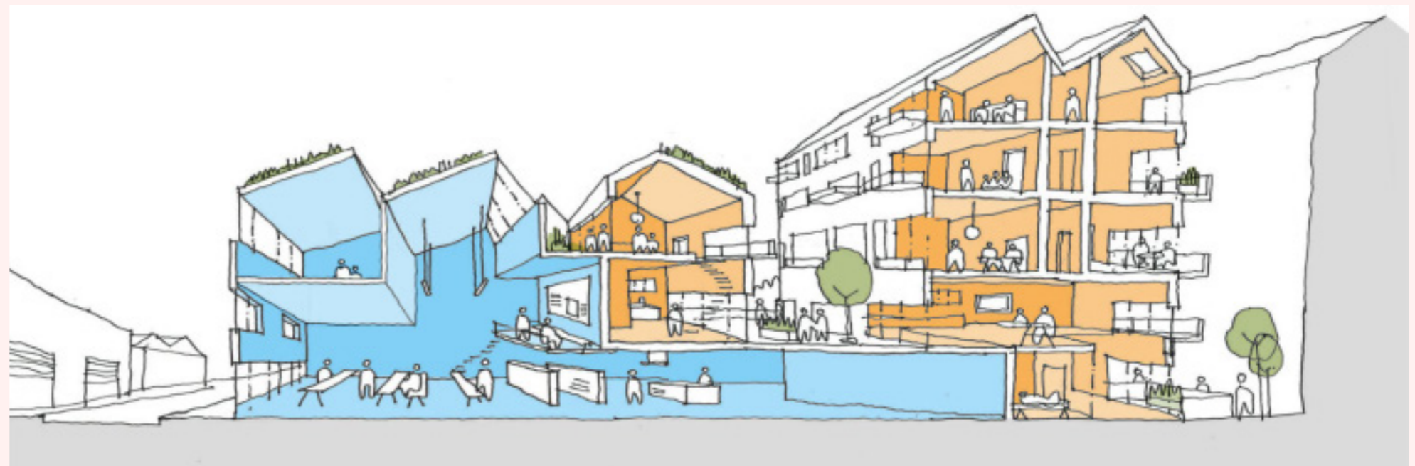
Fig. 22 - Wick Lane, concept sketch of the architectural noise buffer and set back residencies
