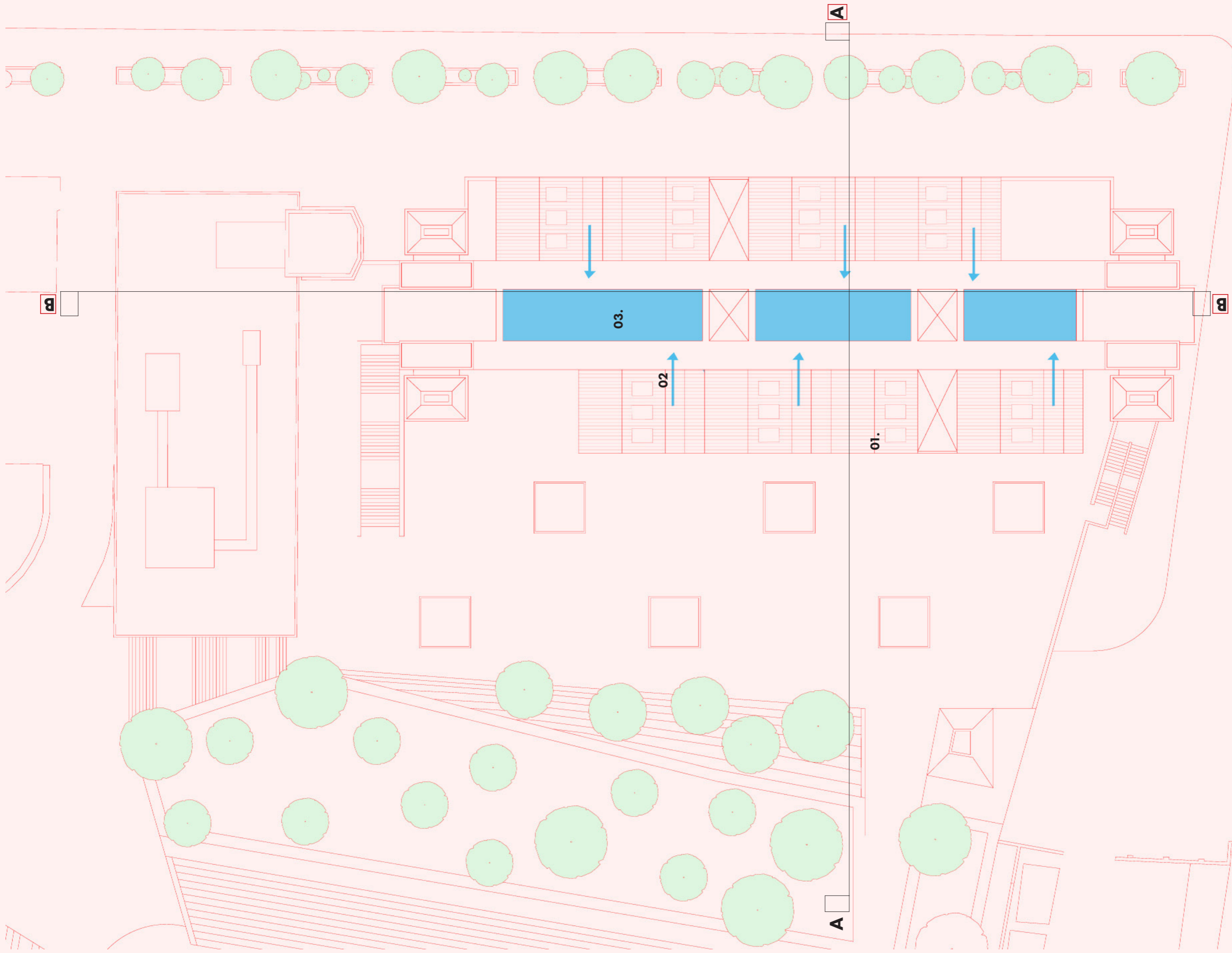
04 (B) - ROOF PLAN - RAINWATER HARVESTING
