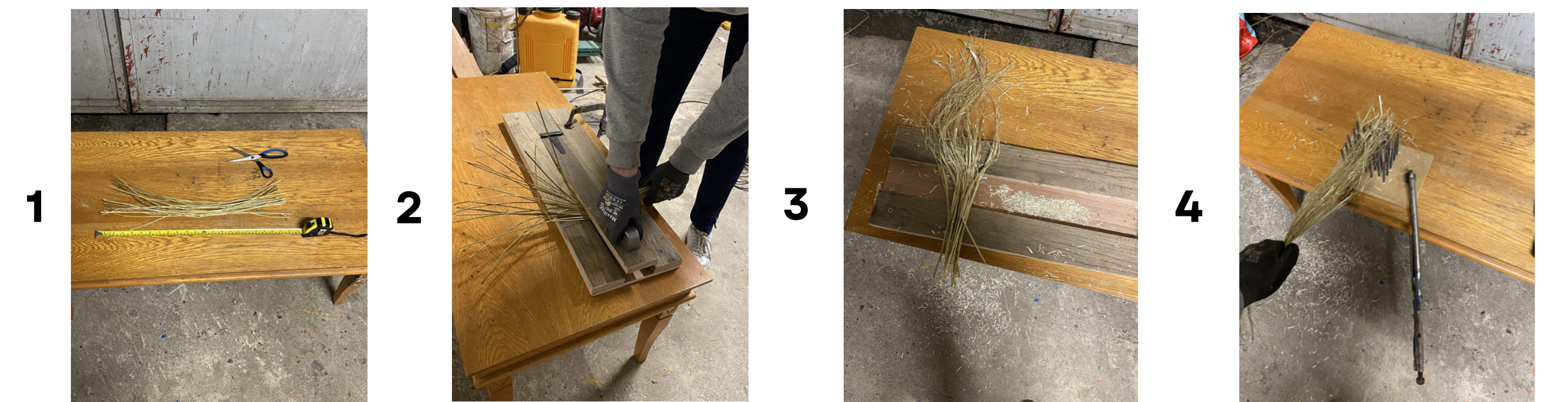
The root and flower part of the plant were cut off initially. The hemp stalks were then broken up and the largest amount of hurd is removed. The stalks are then combed to remove the finer pieces of hurd.
