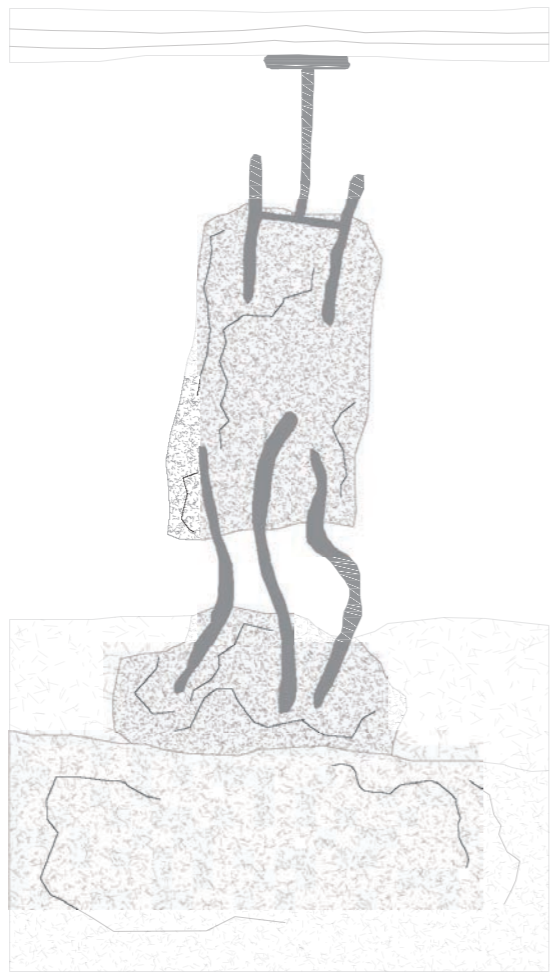
Figure 172 : Stone resting on rebar element. Steel member fixed to stone. Timber walkway as surface level.
