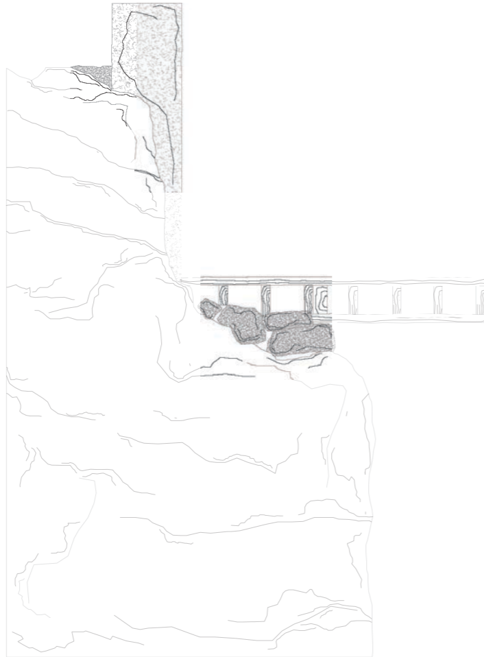
Figure 166 : Low concrete wall cast onto protruding stone. Timber deck resting on concrete.
