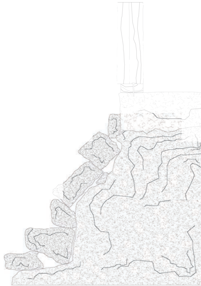
Figure 168 : Stone Laid Diagonally on Protruding Rock Outcropping. Concrete Foundation Cast onto Rock. Timber Rail fixed to Concrete.
